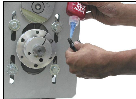
Figure 28 - Install Bushing Hardware
